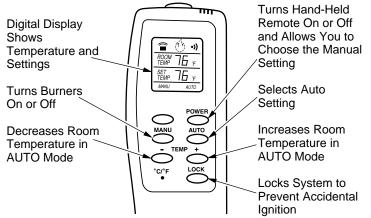
Figure 55 - Thermostat Hand-Held Remote Control Unit Selections (C)GHRCTB
